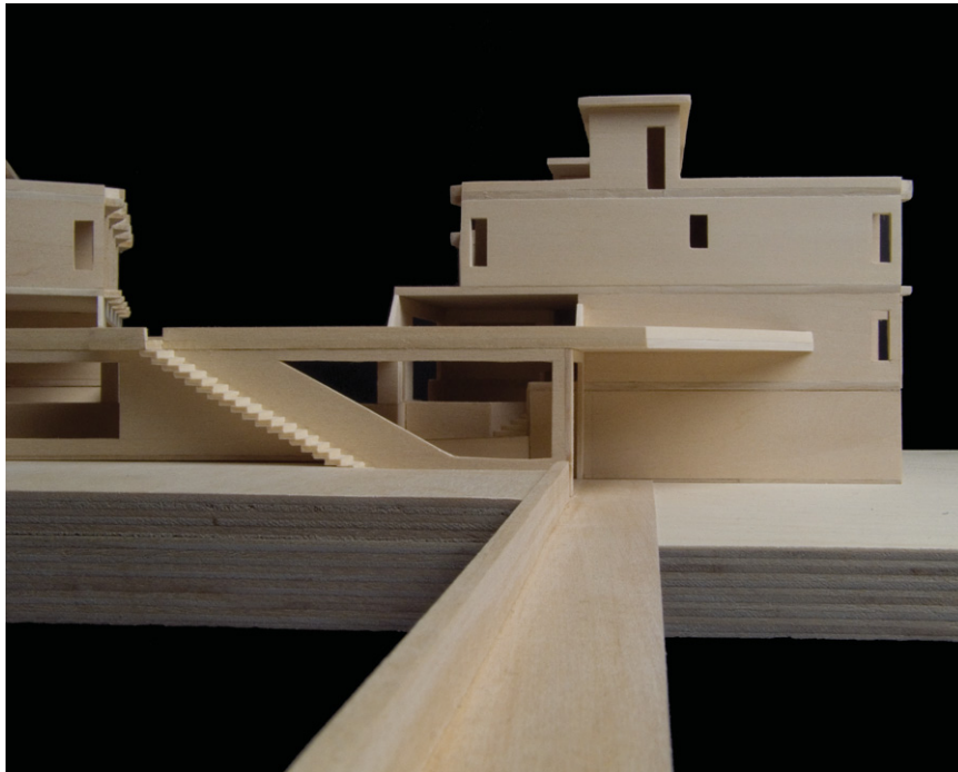
Figure 26 Partial housing model. The path that connects the housing to the main path network is marked by a low stone wall to establish a public address. The entrance is in the one story hinge section that connects the two unit wings as well as offering a transition between the residents and the larger public.
