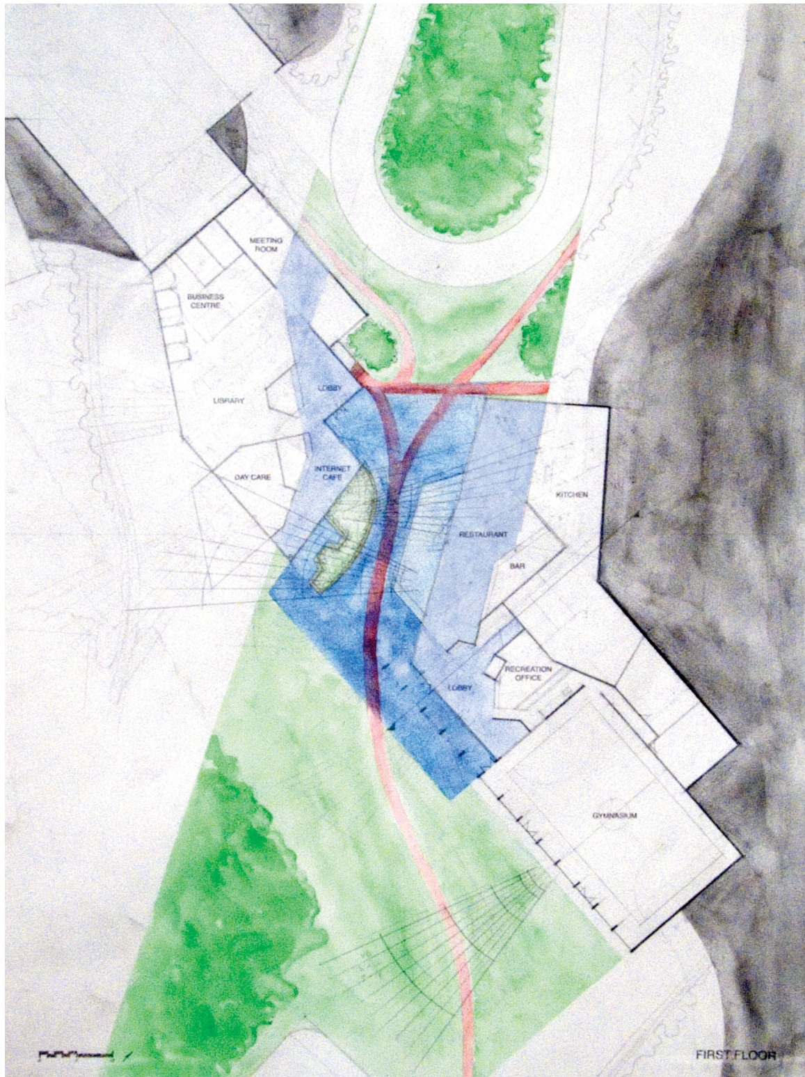
Figure 59 Community Centre first floor plan. The most social spaces of the two buildings, the Internet cafe and the restaurant, face one another across the central civic space and extend into it in nicer weather. Interior spaces are organized to correspond with the exterior surroundings as well as the activities of the adjacent rooms. The gymnasium opens onto the playing fields and looks out at Temple Mountain beyond. The daycare has an adjoining playground and is near the library to facilitate the children's learning.
