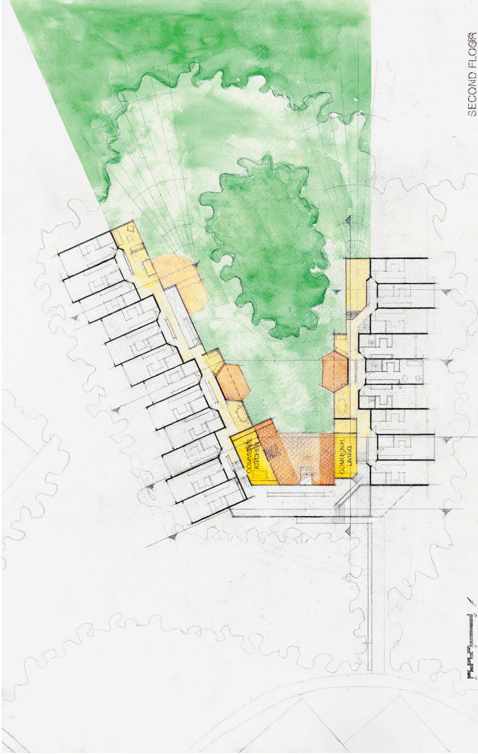
Figure 45 Housing second floor plan. The second floor is designed to accommodate the majority of the activity and nurture the sense of community. A combination of interior and exterior spaces flow into each other to offer a gradient of privacy levels for various interactions. The communal kitchen and living area both continue into the same section of courtyard at grade to create a combined barbecue gathering space. A few steps above, the single circulation space of each wing incorporates living and dining areas overlooking the courtyard, and groupings of entrances to all the units. Inside each unit the kitchen and sitting areas look outward to the adjacent forest and stairs leading up or down to the bedrooms.
