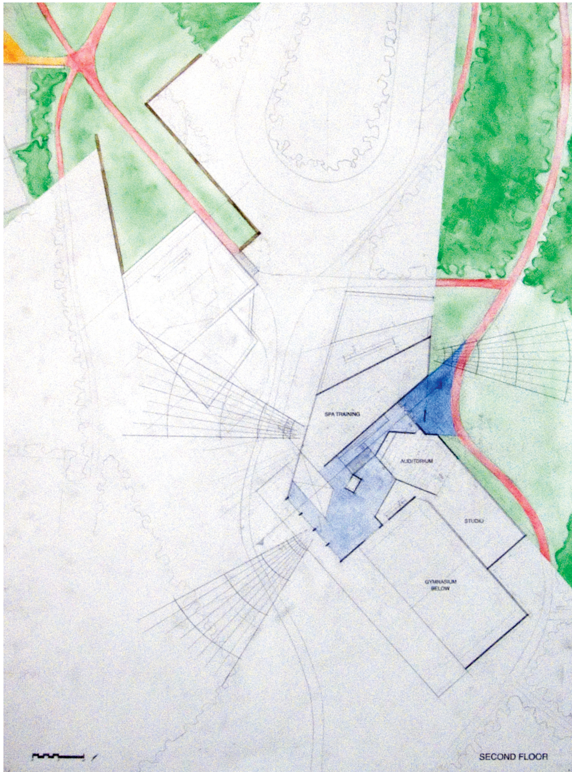
Figure 60 Community Centre second floor plan. Paths from the housing to the east lead to the upper level entrance into the two-story lobby. The studio overlooks the gymnasium and out toward the housing, and is connected to the auditorium as a stage. The spa training facility has views of the glacier and mountains encircling the lake as well as the ski slopes. Residents coming for the western housing follow the path over the roof and down into the civic space between the buildings.
