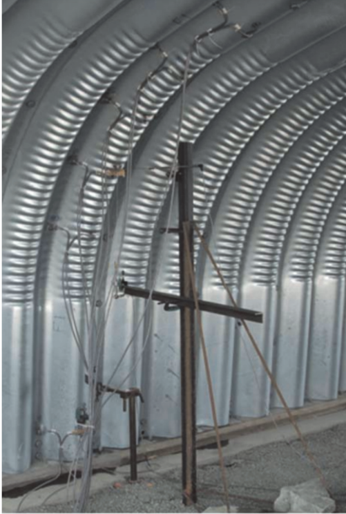
Figure. 3.3 Strain gauges and the displacement measurements at the corrugated haunch area; LVDT for the 14 m span structure
