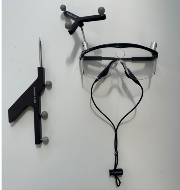
Figure 12. TMS glasses and pointer for co-registration
