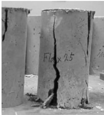
Flax Fiber Reinforced Concrete (Fernandez 2012)
