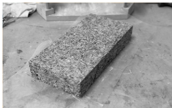
Flaxcrete block made by author for The Flaxmobile Farmers Retreat (Recipe from Garikapati et al. 2020)
