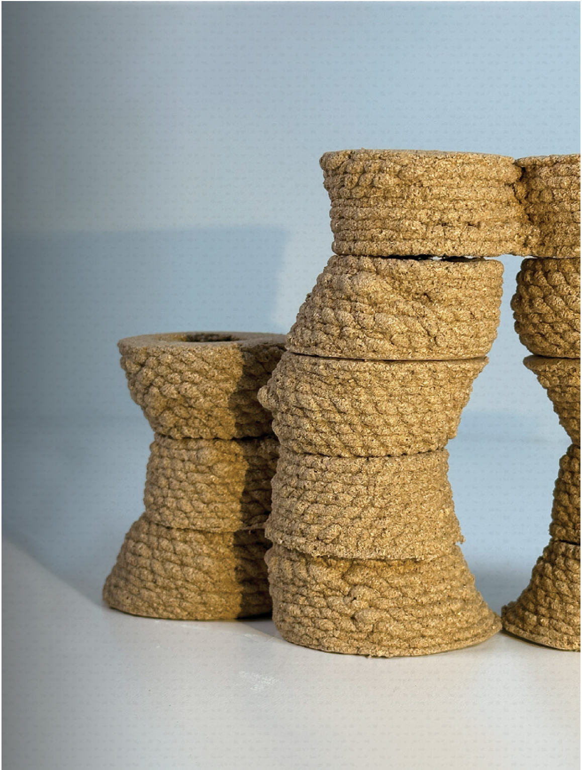
Assembled permeable wall set up
