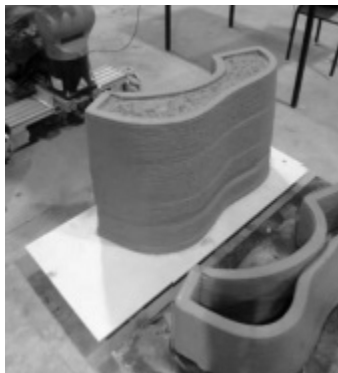
Image of printed concrete containing shives. (Dubois et al. 2018)
