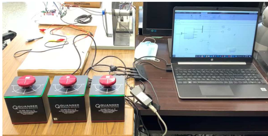
Figure 12.7: Experimental setup to test improved CSC architecture on multilateral teleoperation system
