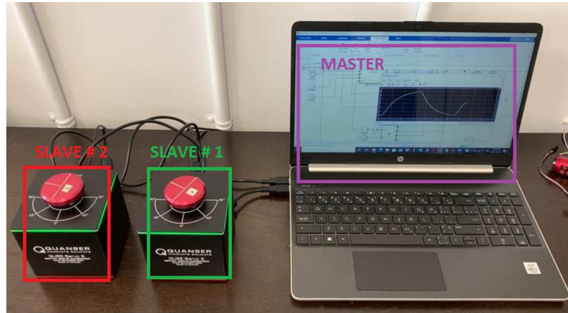
Figure 5.12: Experimental setup to test asymmetric teleoperation system (ATS)
