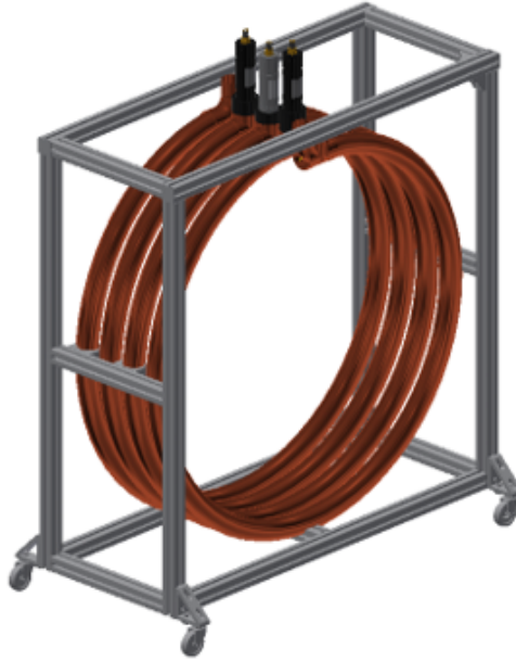
Figure 3.1: 3D rendering of the hydrophone calibration system. The projector is located in the middle with the two hydrophones on either side.
