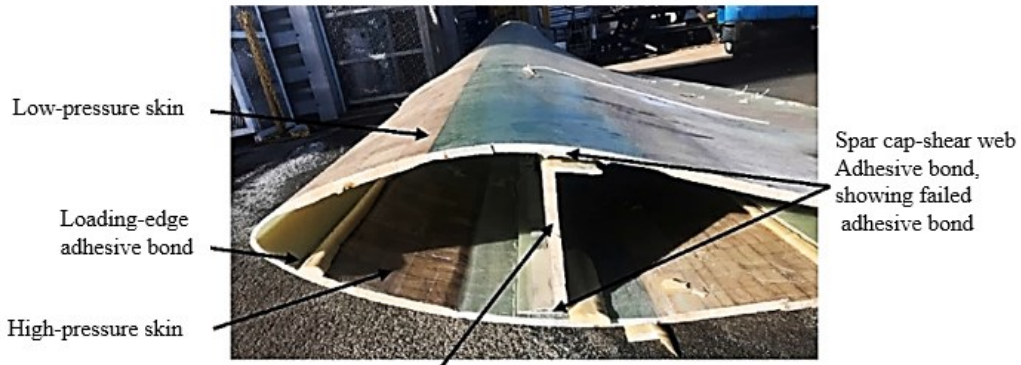
Figure 1-14. Cross-section of Sandia National Laboratories' National Rotor Testbed 13-m blade, showing the ABJ parts (Murray et al., 2019).
