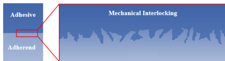
Figure 1-6. Mechanical interlocking facilitates the flow of the adhesive into the morphological irregularities of an adherend's surface.
