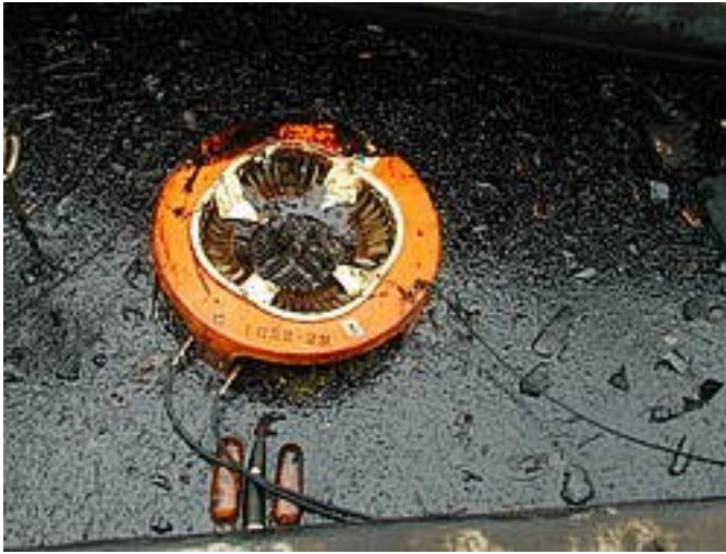
Figure 5 An image example of a small skimmer being used (Use of Skimmers in Oil Pollution Response, 2014)
