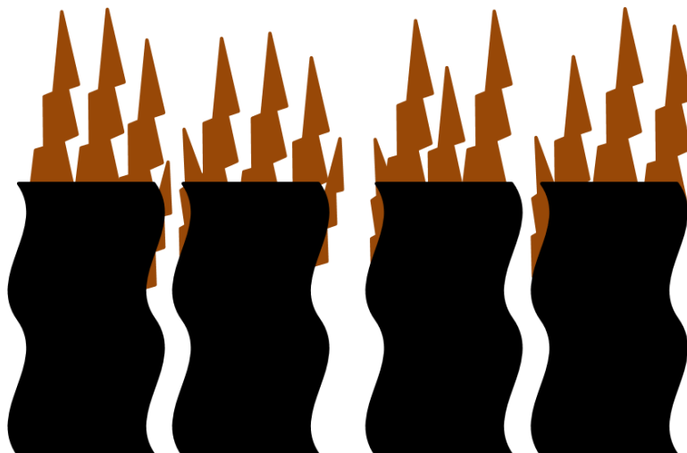
Figure 6-5. Hypothetical physical configuration of electrodeposited manganese oxide on porous carbon.
