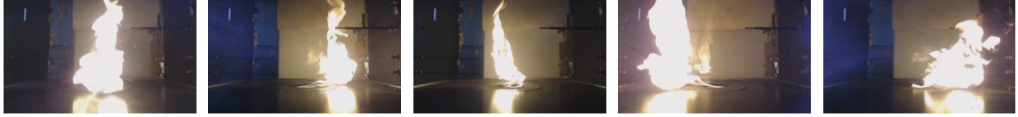
(a) Example of tilting— i.e. , the transformation of horizontal vorticity into vertical vorticity and vice versa .
