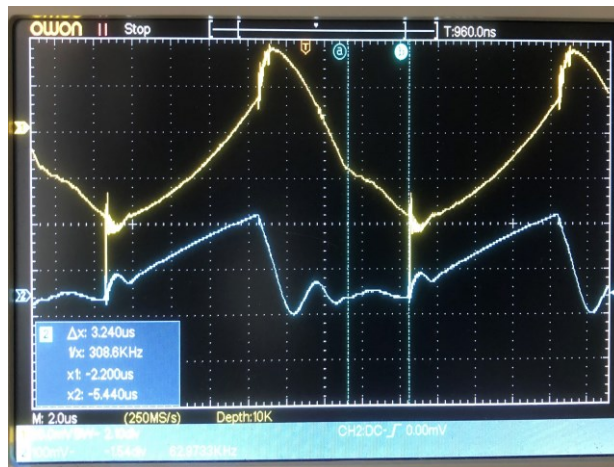
Fig .72. Inductor currents, I_{L1} , (top) and I_{L2} , (bottom) [80] 2022 IEEE.
