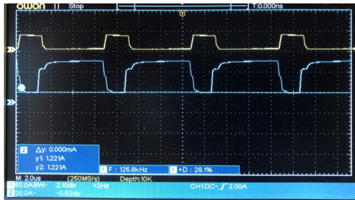
Fig. 85. The voltage of node A with respect to gate pulse (top), in the interleaved method with no phase shift.
