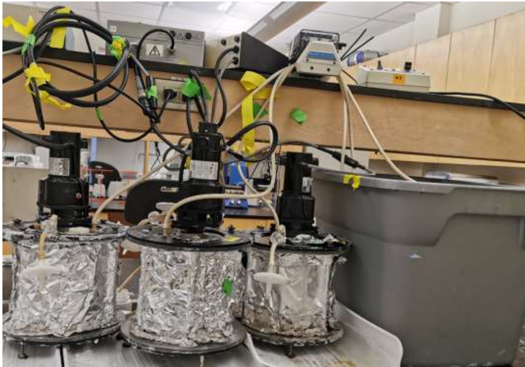
Figure 4.1 Experimental set-up. AR1 (left) tested coupons with GC111 formula. AR2 (middle) tested coupons with GC112 formula. AR3(right) tested uncoated coupons.
