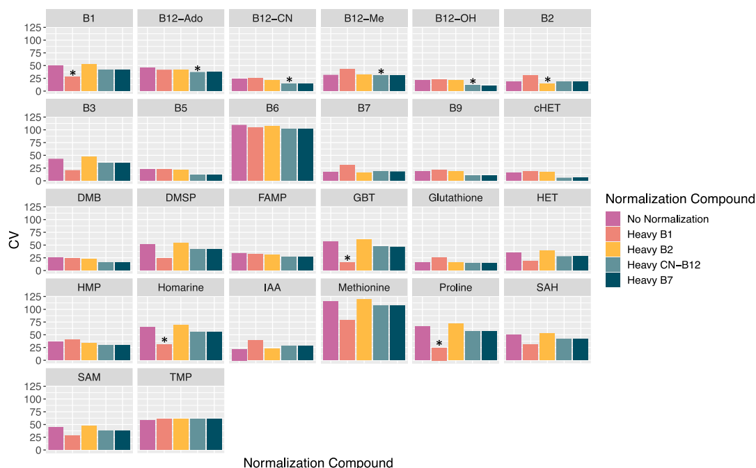
Figure S3.4: The effects of different normalizations on the coefficient of variation (CV) among quality control (QC) samples injected periodically during the metabolite analysis run. Normalizations which reduced QC CV by more than 10% were chosen as the best matched internal standard (BMIS) for that compound. The chosen BMIS is marked for each compound with a star. If no star is included, the compounds was not normalized to a BMIS.
