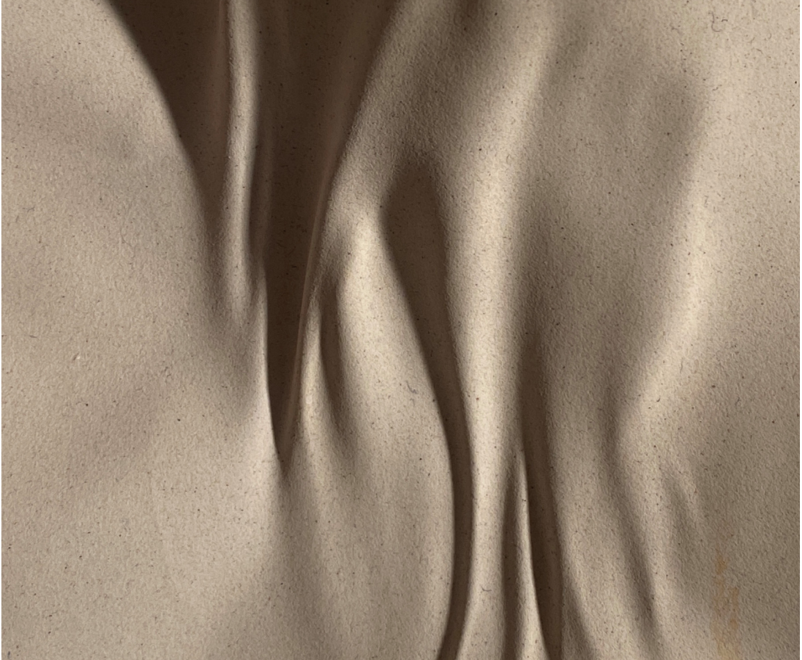
Close up of materially induced warping patterns in carrageenan calcium carbonate membrane.
