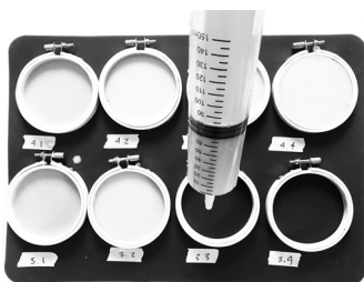
Pouring solution into formwork.
