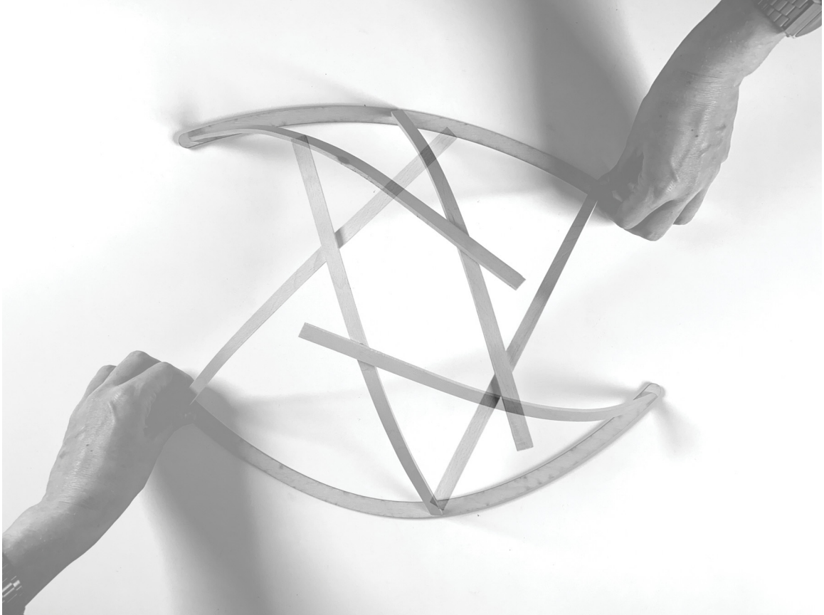
The structure of gradient scales pavilion is comprised of steam-bent beech.
