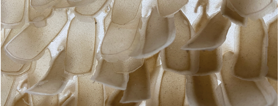
Detail of gradient scales model showing variable translucency as a function of calcium carbonate.
