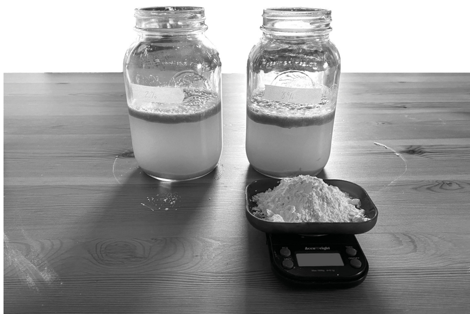
Mixing protocol process: hydrating carrageenan and calcium carbonate with water.
