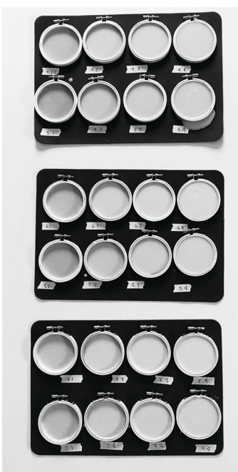
Membranes drying in formwork.
