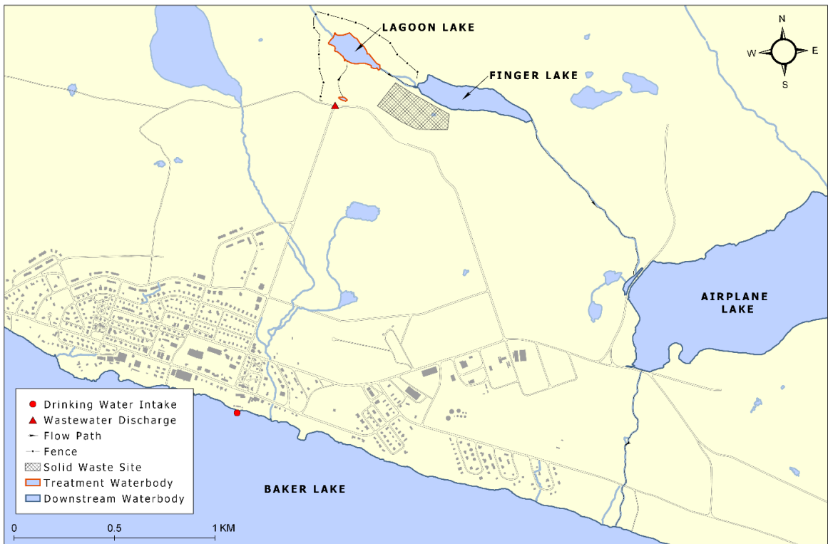
Figure 3.2.3 Watershed treatment process and flow path
