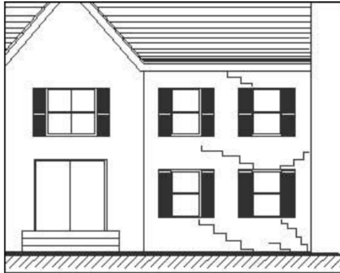
Figure 2.5: Cracks caused due to the settlement of Marine clay deposits (Fairfax County publication)
