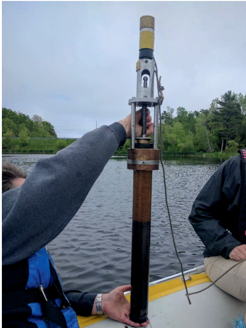
Figure A.6 Gravity corer device (Photograph taken on May 17, 2018).
