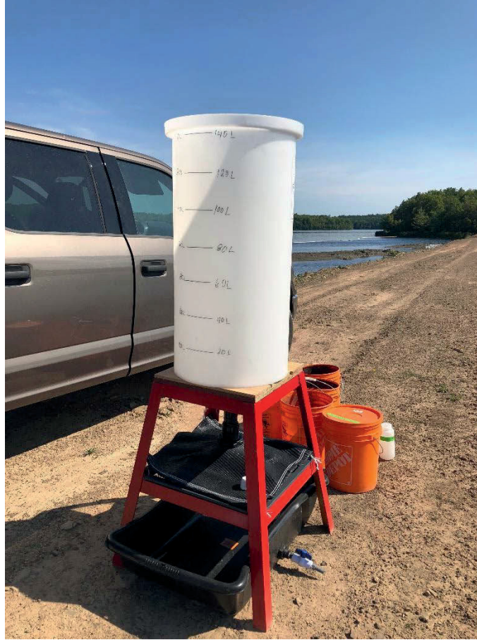
Figure 5.1 Geotube Dewatering Test (GDT) Setup (Photograph taken on December 6, 2018)
