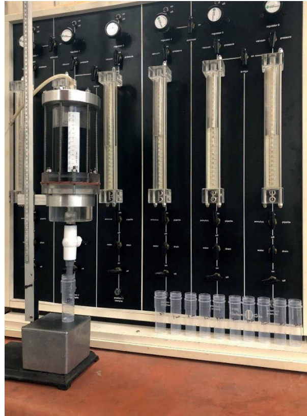
Figure 6.1 Pressure Filtration Test (PFT) (a) cell, (b) setup
