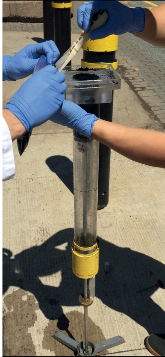
Figure A.7 Gravity core extruder apparatus (Photograph taken on July 7, 2017)
