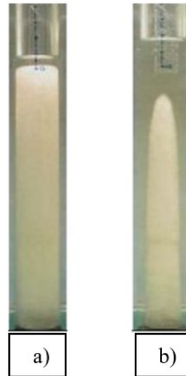
Figure 2.3 Melting of RT27 in a vertical cylinder of 3 cm diameter and a melting temperature differential of 10 °C at a) t = 4 min and b) t = 28 min (Shmueli et al. , 2010).
