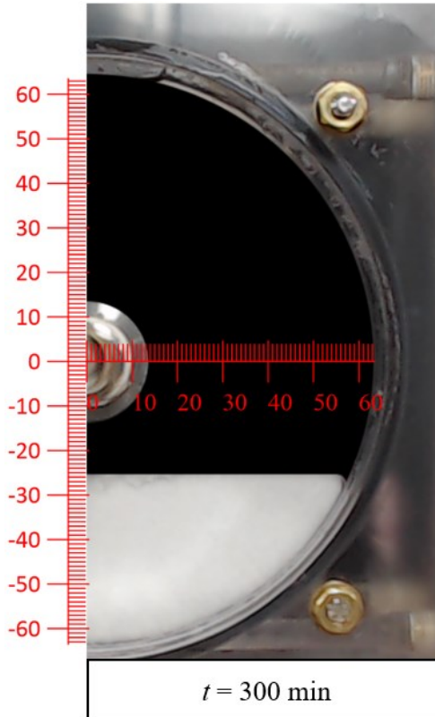
Figure 4.5 Physical measurement of melt thickness for melting of n -octadecane in the enclosure with the center-tube diameter of 27 mm for \Delta T_f = 25.3 °C and \Delta T_s = 7.5 °C using the front face as the reference.
