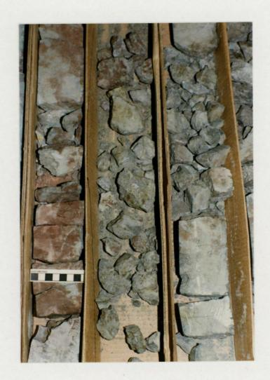
Plate 12: Silty shale and argillaceous siltstone rubble: very friable and soft with slickensides and red staining. 3892 m, core 9, Hibernia K-14.
