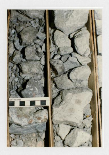
Plate 11: Fault breccia (below scale) with sideritic pebbles in clay-rich, slickensided rubble. 3910 m, core 10, Hibernia B-27.
