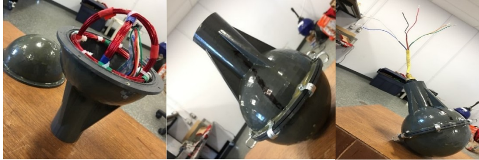
Figure 25: Adding connector cables and sealing with epoxy
