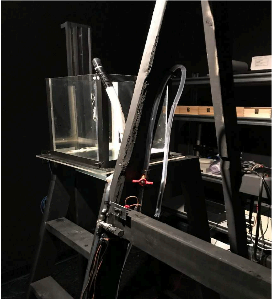
Figure 10 Actual Experimental lab setup while taking measurements with HyperOCR 444 Radiance sensor.
