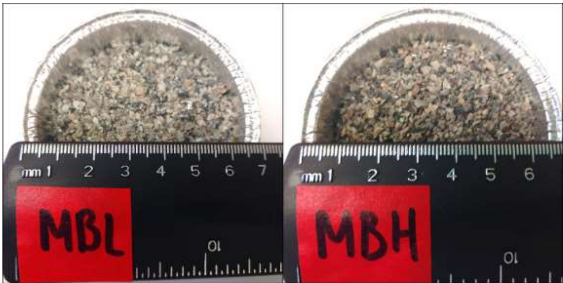
Figure B-3: Millet Brook granite. Sampled from the DNR Core Library (drill hole MB 80 C2-1, 37.7 to 41.8 m depth, Aquitaine Company of Canada, Ltd.).
