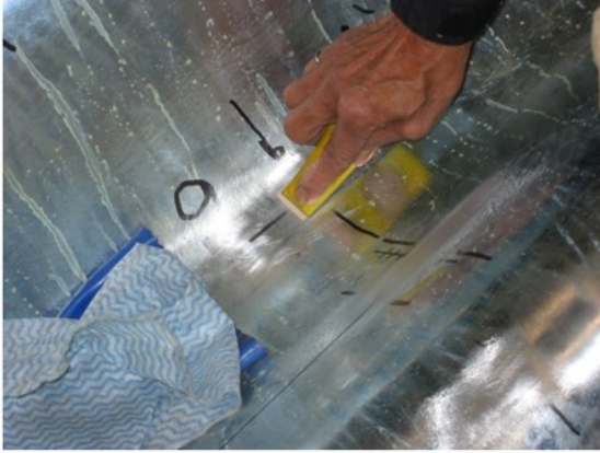
Figure 4-17: a) Removing galvanizing b) bonding strain gauge to plate
