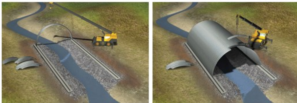
Figure 4-6: Placement of first ring, sub-component assembly
