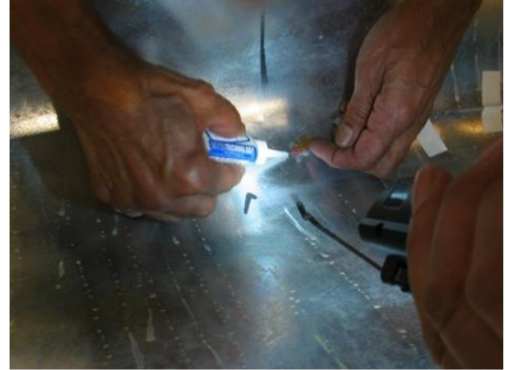
Figure 4-17: a) Removing galvanizing b) bonding strain gauge to plate
