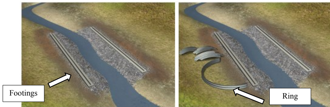
Figure 4-5: Footing with base channel installation, first ring assembly
