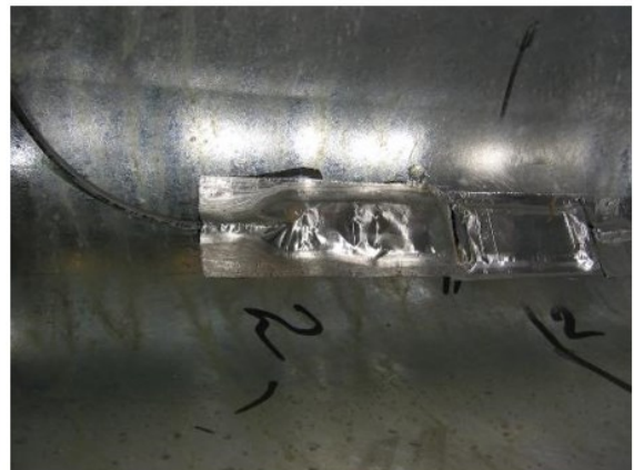
Figure 4-18: a) Applying butyl rubber b) gauge with foil cover and temp gauge
