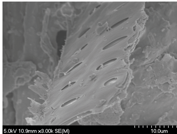
Figure 47 Scanning Electron Microscope Picture of Poplar Wood (45-75 \mu\text{m} ) Torrefied at 300 ^{\circ}\text{C} Showing Pore Openings
