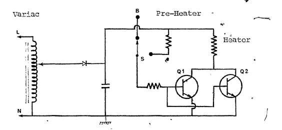
Fig. 51. Block Diagram of the Black-Body Control Circuit.
