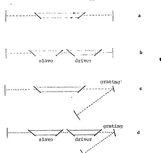
Fig. 3. Cavities of chemical lasers employed for vibrational population distributions
