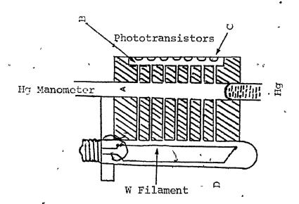
Phototransistor Device for Flow Pate Measurements. 52 Fig
