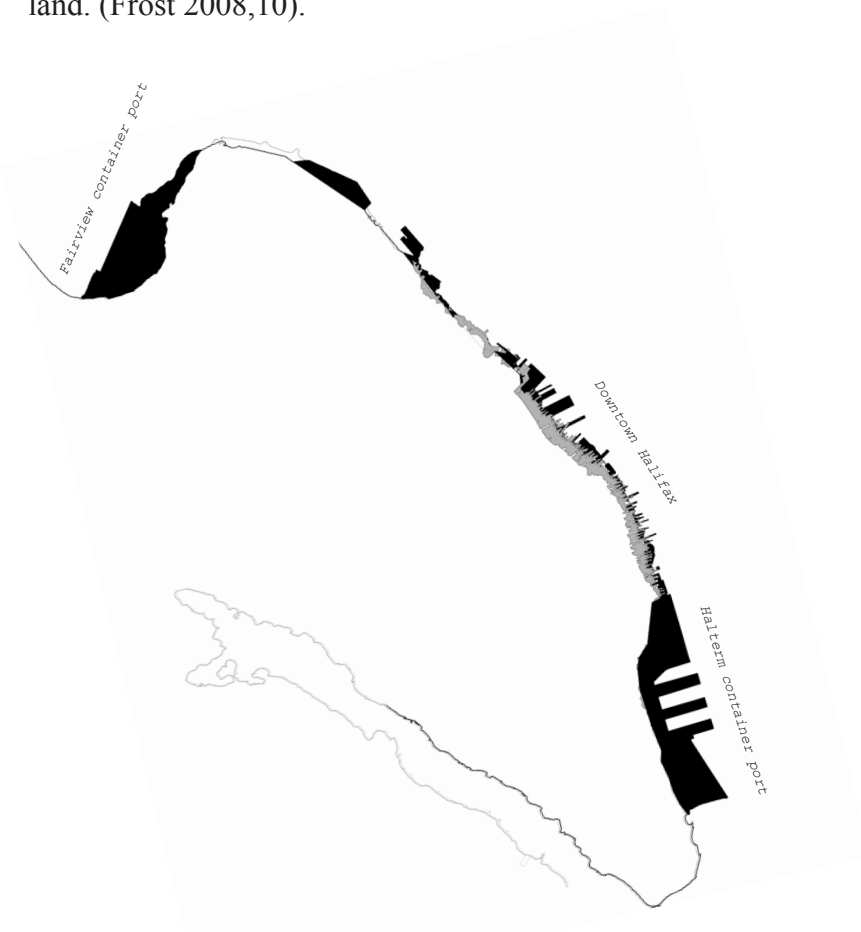
Infill diagram on the Halifax Peninsula. Original landform in white, 1865 coastal infill in grey, current coastal infill in black.
