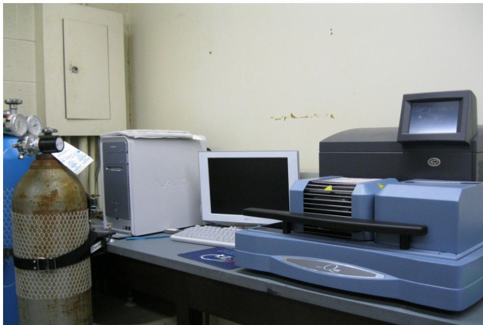
Figure 3.2 Thermal Gravimetric Analyzer Apparatus (TGA).
