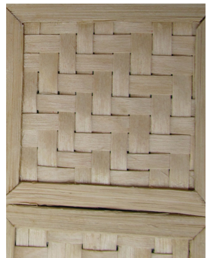
Photograph of model of woven cladding panel. Lightweight panels are easy to transport, employ local skill from textile industry (the second largest industry in the country), and their fabrication recognizes the abundance of time and skilled workers available.
