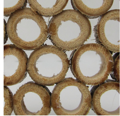
Photograph of model of cladding panel made with off-cuts of bamboo. These panels provide ventilation and allow day lighting. They are located on inset walls for protection from weather.
