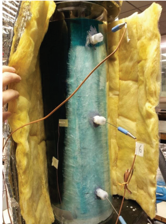
Figure 6.3: Photograph of LHESS after 24 hours of simultaneous charging/discharging at 2.75 L/min
