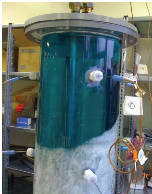
Figure 5.5: Photograph of system charging after 20 hours (no insulation for observation)
