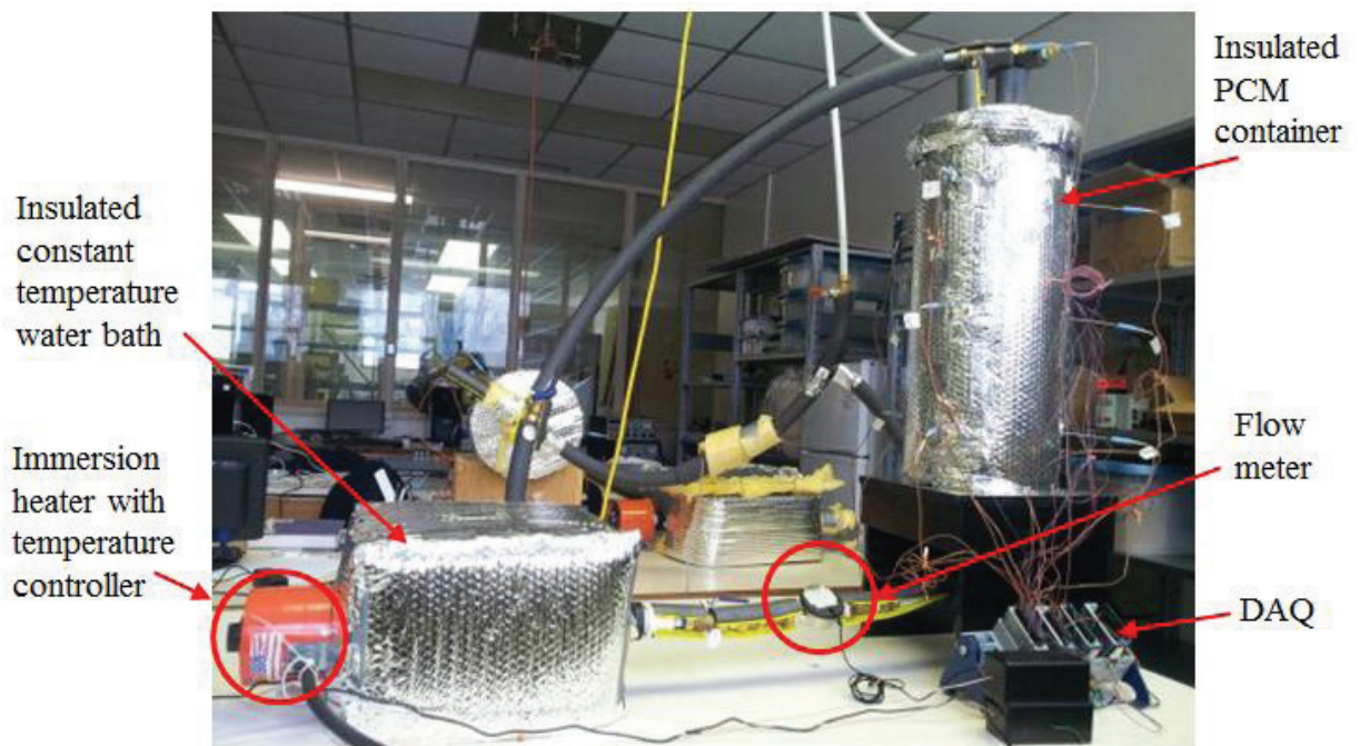
Figure 3.6: Experimental setup including PCM container, hot water bath, flow meter, and DAQ (Another LHESS experimental setup is seen in the background)
