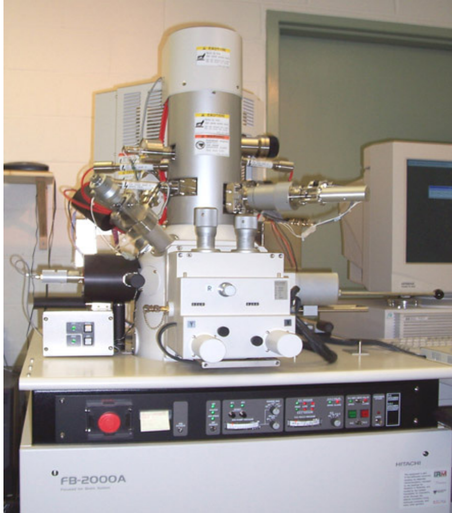
Figure 45: Front View of Focused Ion Beam (FIB) Instrument Used for Etching [25]
