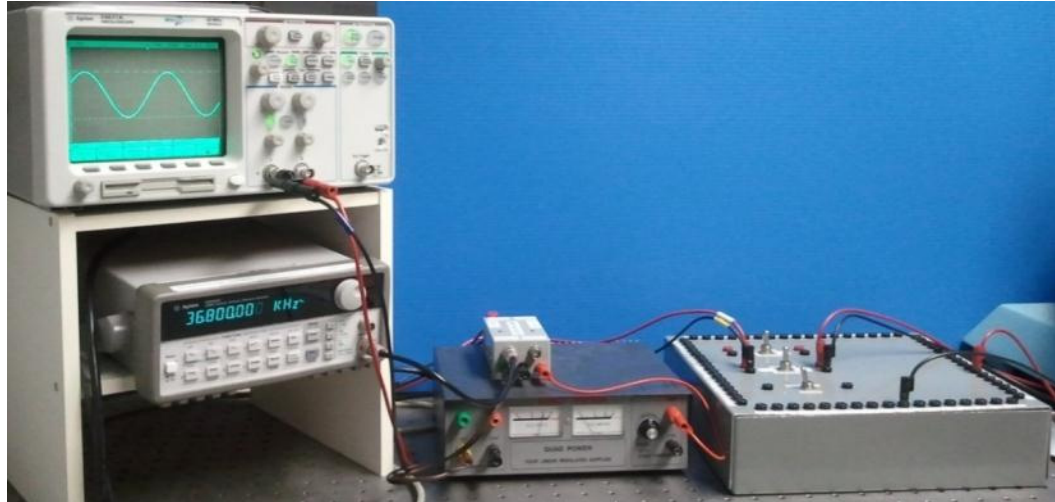
Figure 41: Part of Micro Scale Setup Including: Oscilloscope, Function Generator, Amplifier with its Power Supply and Distribution Box
