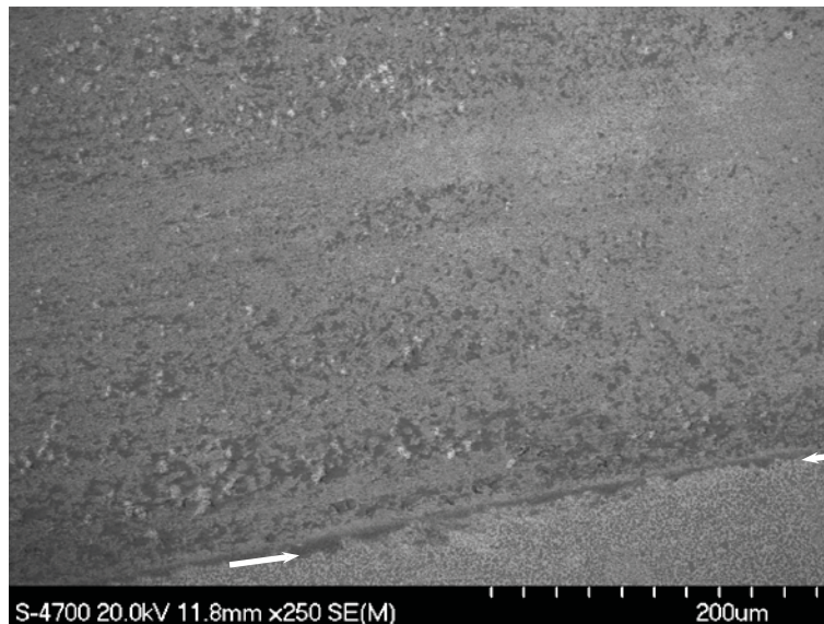
Figure 55. SEM image of the wear track edge for a \text{Ti}(\text{C}_{0.7},\text{N}_{0.3}) sample, prepared with 40 vol. % \text{Ni}_3\text{Al} , demonstrating minimal deformation outside of the wear track (nominal reciprocating direction left to right).
