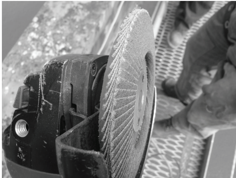
Figure 8-4 : Grinder and sanding wheel in field
