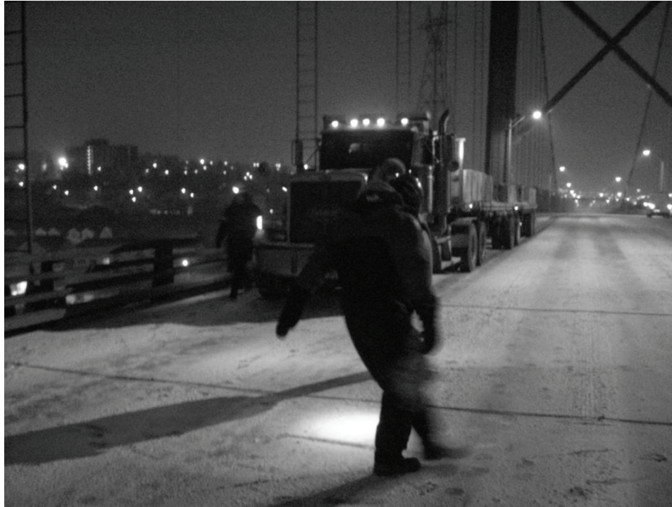
Figure 7-6 : Positioning of calibration truck for static testing
