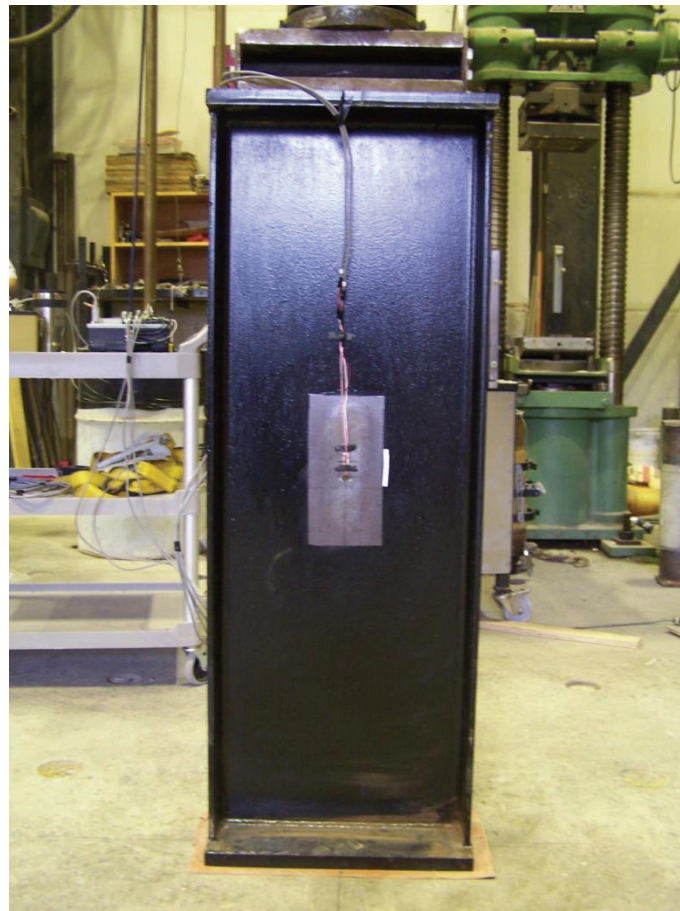
Figure 6-5 : Full-scale laboratory compression test specimen
