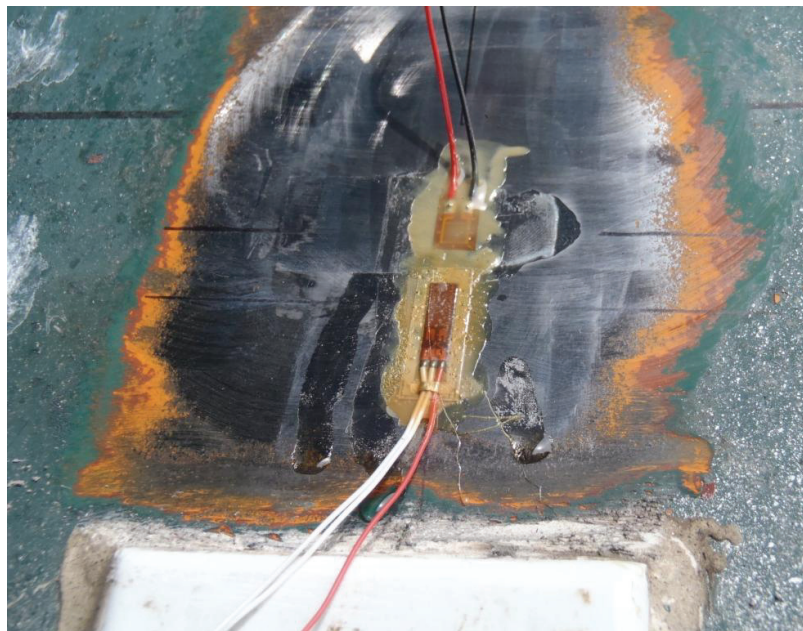
Figure 6-8 : Gauge type comparison - bridge member
