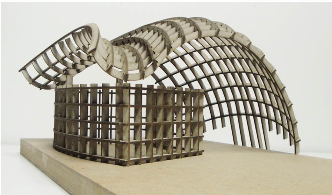
fig. 53. Models showing geometry of the Vaulted roof forms
