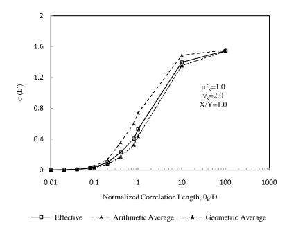
Figure 4.21: Influence of correlation length on the standard deviation of effective hydraulic conductivity for a coefficient of variation of 2.0 and an aspect ratio of liner of 1.0
