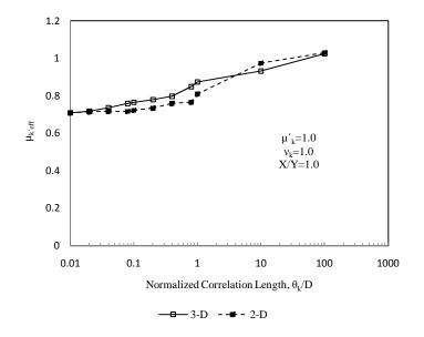
Figure B.3: Comparison between 3-D and 2-D mean of effective hydraulic conductivity for aspect ratio of liner of 1.0
