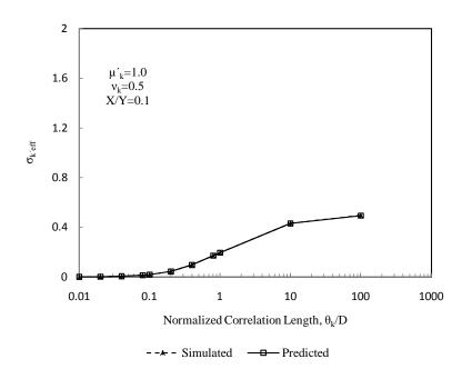
Figure 4.25: Comparison between simulated and predicted standard deviation of effective hydraulic conductivity for a coefficient of variation of 0.5 and aspect ratio of liner of 0.1
