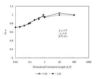
Figure B.1: Comparison between 3-D and 2-D mean of effective hydraulic conductivity for aspect ratio of liner of 0.1
