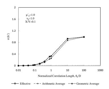
Figure 4.15: Influence of correlation length on the standard deviation of effective hydraulic conductivity for a coefficient of variation of 1.0 and an aspect ratio of liner of 0.1
