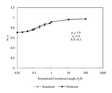
Figure 4.9: Comparison between simulated and predicted mean of effective hydraulic conductivity for a coefficient of variation of 1.0 and an aspect ratio of liner of 0.3
