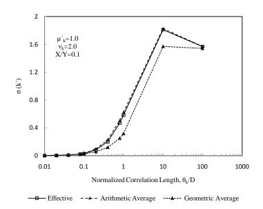
Figure 4.20: Influence of correlation length on the standard deviation of effective hydraulic conductivity for a coefficient of variation of 2.0 and an aspect ratio of liner of 0.1
