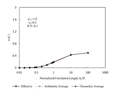
Figure 4.18: Influence of correlation length on the standard deviation of effective hydraulic conductivity for a coefficient of variation of 0.5 and an aspect ratio of liner of 0.1
