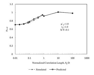
Figure 4.8: Comparison between simulated and predicted mean of effective hydraulic conductivity for a coefficient of variation of 1.0 and an aspect ratio of liner of 0.1
