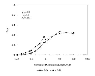
Figure B.4: Comparison between 3-D and 2-D standard deviation of effective hydraulic conductivity for aspect ratio of liner of 0.1
