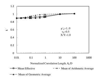
Figure 4.5: Influence of correlation length on the mean of effective hydraulic conductivity for a coefficient of variation of 0.5 and an aspect ratio of liner of 1.0
