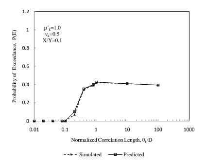
Figure 4.32: Comparison between simulated and predicted probability of exceedance for a coefficient of variation of 0.5 and an aspect ratio of liner of 0.1
