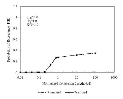
Figure 4.31: Comparison between simulated and predicted probability of exceedance for a coefficient of variation of 1.0 and aspect ratio of liner of 1.0
