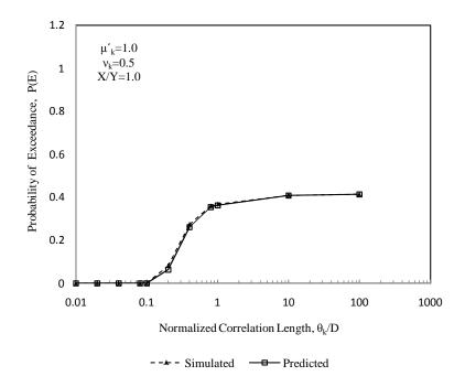
Figure 4.33: Comparison between simulated and predicted probability of exceedance for a coefficient of variation of 0.5 and aspect ratio of liner of 1.0
