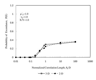
Figure 4.44: Comparison between 3-D and 2-D probability of exceedance for aspect ratio of liner of 1.0
