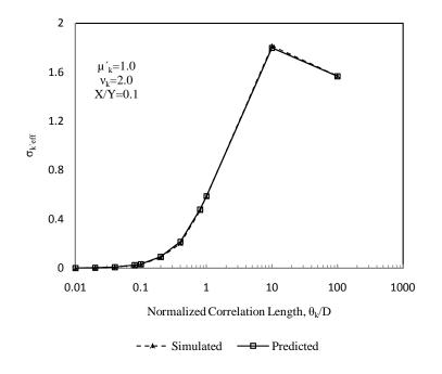
Figure 4.27: Comparison between simulated and predicted standard deviation of effective hydraulic conductivity for a coefficient of variation of 2.0 and an aspect ratio of liner of 0.1
