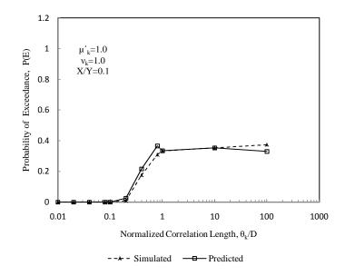
Figure 4.29: Comparison between simulated and predicted probability of exceedance for a coefficient of variation of 1.0 and an aspect ratio of liner of 0.1
