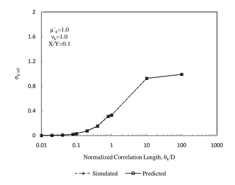
Figure 4.22: Comparison between simulated and predicted standard deviation of effective hydraulic conductivity for a coefficient of variation of 1.0 and an aspect ratio of liner of 0.1
