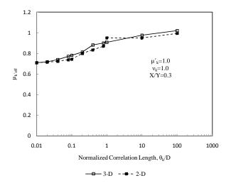
Figure B.2: Comparison between 3-D and 2-D mean of effective hydraulic conductivity for aspect ratio of liner of 0.3
