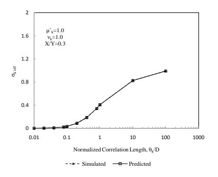
Figure 4.23: Comparison between simulated and predicted standard deviation of effective hydraulic conductivity for a coefficient of variation of 1.0 and an aspect ratio of liner of 0.3
