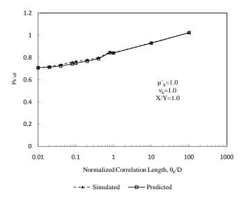
Figure 4.10: Comparison between simulated and predicted mean of effective hydraulic conductivity for a coefficient of variation of 1.0 and an aspect ratio of liner of 1.0
