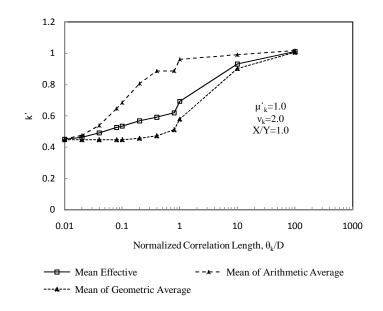
Figure 4.7: Influence of correlation length on the mean of effective hydraulic conductivity for a coefficient of variation of 2.0 and an aspect ratio of liner of 1.0
