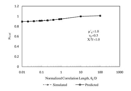
Figure 4.12: Comparison between simulated and predicted mean of effective hydraulic conductivity for a coefficient of variation of 0.5 and an aspect ratio of liner of 1.0
