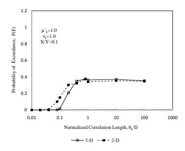
Figure 4.42: Comparison between 3-D and 2-D probability of exceedance for aspect ratio of liner of 0.1
