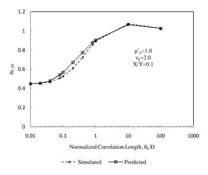
Figure 4.13: Comparison between simulated and predicted mean of effective hydraulic conductivity for a coefficient of variation of 2.0 and an aspect ratio of liner of 0.1
