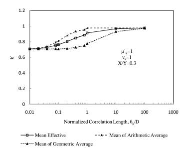
Figure 4.2: Influence of correlation length on the mean of effective hydraulic conductivity for a coefficient of variation of 1.0 and an aspect ratio of liner of 0.3
