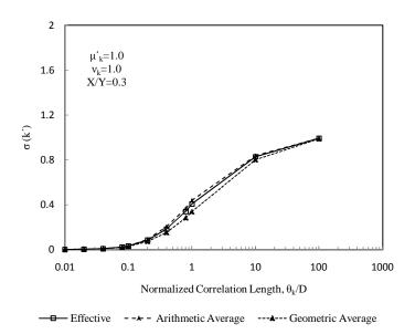
Figure 4.16: Influence of correlation length on the standard deviation of effective hydraulic conductivity for a coefficient of variation of 1.0 and an aspect ratio of liner of 0.3
