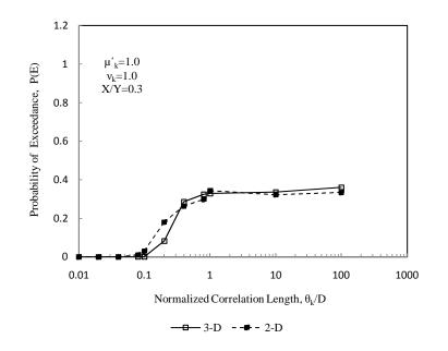
Figure 4.43: Comparison between 3-D and 2-D probability of exceedance for aspect ratio of liner of 0.3
