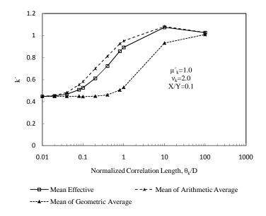
Figure 4.6: Influence of correlation length on the mean of effective hydraulic conductivity for a coefficient of variation of 2.0 and an aspect ratio of liner of 0.1
