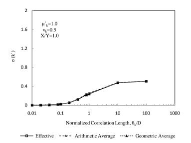
Figure 4.19: Influence of correlation length on the standard deviation of effective hydraulic conductivity for a coefficient of variation of 0.5 and an aspect ratio of liner of 1.0
