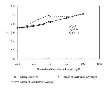
Figure 4.3: Influence of correlation length on the mean of effective hydraulic conductivity for a coefficient of variation of 1.0 and an aspect ratio of liner of 1.0
