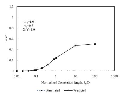
Figure 4.26: Comparison between simulated and predicted standard deviation of effective hydraulic conductivity for a coefficient of variation of 0.5 and an aspect ratio of liner of 1.0
