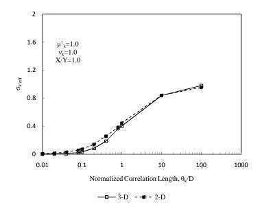
Figure B.6: Comparison between 3-D and 2-D standard deviation of effective hydraulic conductivity for aspect ratio of liner of 1.0
