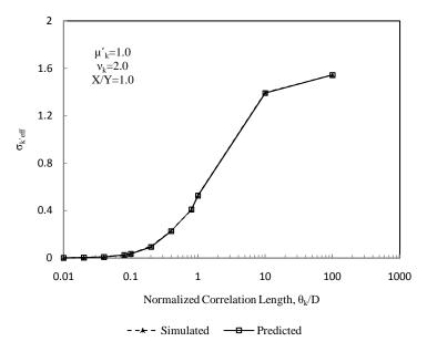
Figure 4.28: Comparison between simulated and predicted standard deviation of effective hydraulic conductivity for a coefficient of variation of 2.0 and an aspect ratio of liner of 1.0
