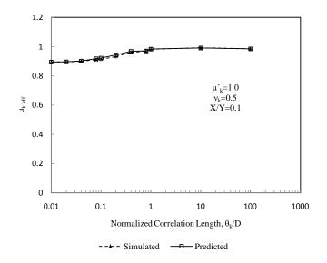
Figure 4.11: Comparison between simulated and predicted mean of effective hydraulic conductivity for a coefficient of variation of 0.5 and an aspect ratio of liner of 0.1
