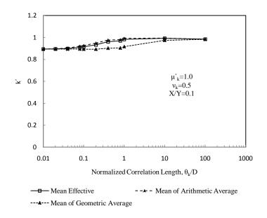
Figure 4.4: Influence of correlation length on the mean of effective Hydraulic conductivity for a coefficient of variation of 0.5 and an aspect ratio of liner of 0.1
