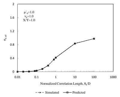
Figure 4.24: Comparison between simulated and predicted standard deviation of effective hydraulic conductivity for a coefficient of variation of 1.0 and an aspect ratio of liner of 1.0
