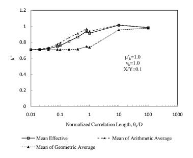
Figure 4.1: Influence of correlation length on the mean of effective hydraulic conductivity for a coefficient of variation of 1.0 and an aspect ratio of liner of 0.1
