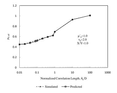
Figure 4.14: Comparison between simulated and predicted mean of effective hydraulic conductivity for a coefficient of variation of 2.0 and an aspect ratio of liner of 1.0
