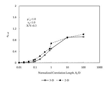
Figure B.5: Comparison between 3-D and 2-D standard deviation of effective hydraulic conductivity for aspect ratio of liner of 0.3
