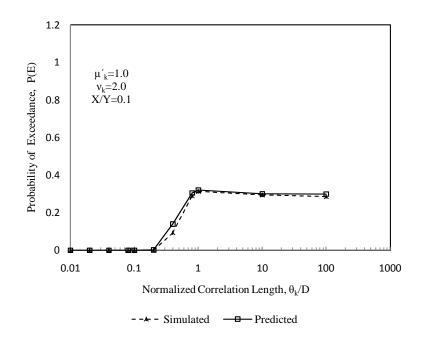
Figure 4.34: Comparison between simulated and predicted probability of exceedance for a coefficient of variation of 2.0 and aspect ratio of liner of 0.1
