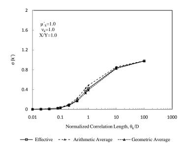
Figure 4.17: Influence of correlation length on the standard deviation of effective hydraulic conductivity for a coefficient of variation of 1.0 and an aspect ratio of liner of 1.0
