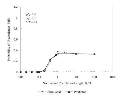
Figure 4.30: Comparison between simulated and predicted probability of exceedance for a coefficient of variation of 1.0 and an aspect ratio of liner of 0.3
