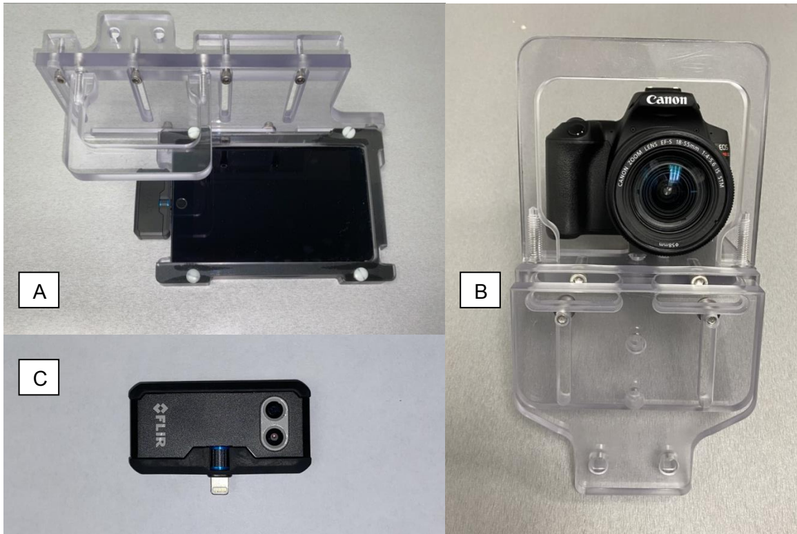
Figure 2.2. (A) The FLIR One Pro camera paired to an iPad, and (B) Canon Rebel SL3 DSLR camera used to acquire thermal and optical images, respectively, bolted to plexiglass camera-holding mounts. (C) A close up view of the FLIR One Pro camera.
