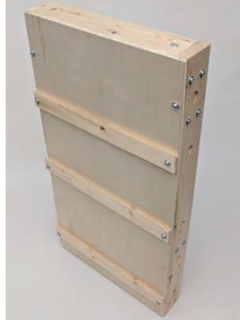
1/4 scale construction details of bolted interior wall panels and attached french cleat hangers
