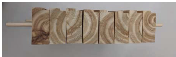
Cedar DLT panels tests with squared edge and facet
