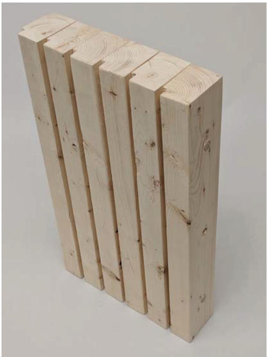
Spruce DLT panels tests with double blade cut and squared edge finish
