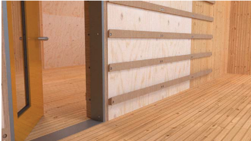
Wall panel with door assembly and french cleats
