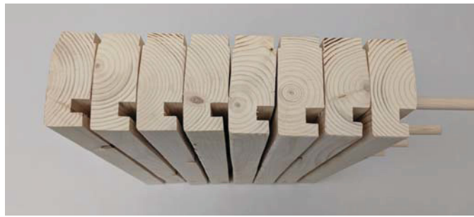
Spruce DLT panels tests with single blade cut and acoustic grooves for sound dampening
