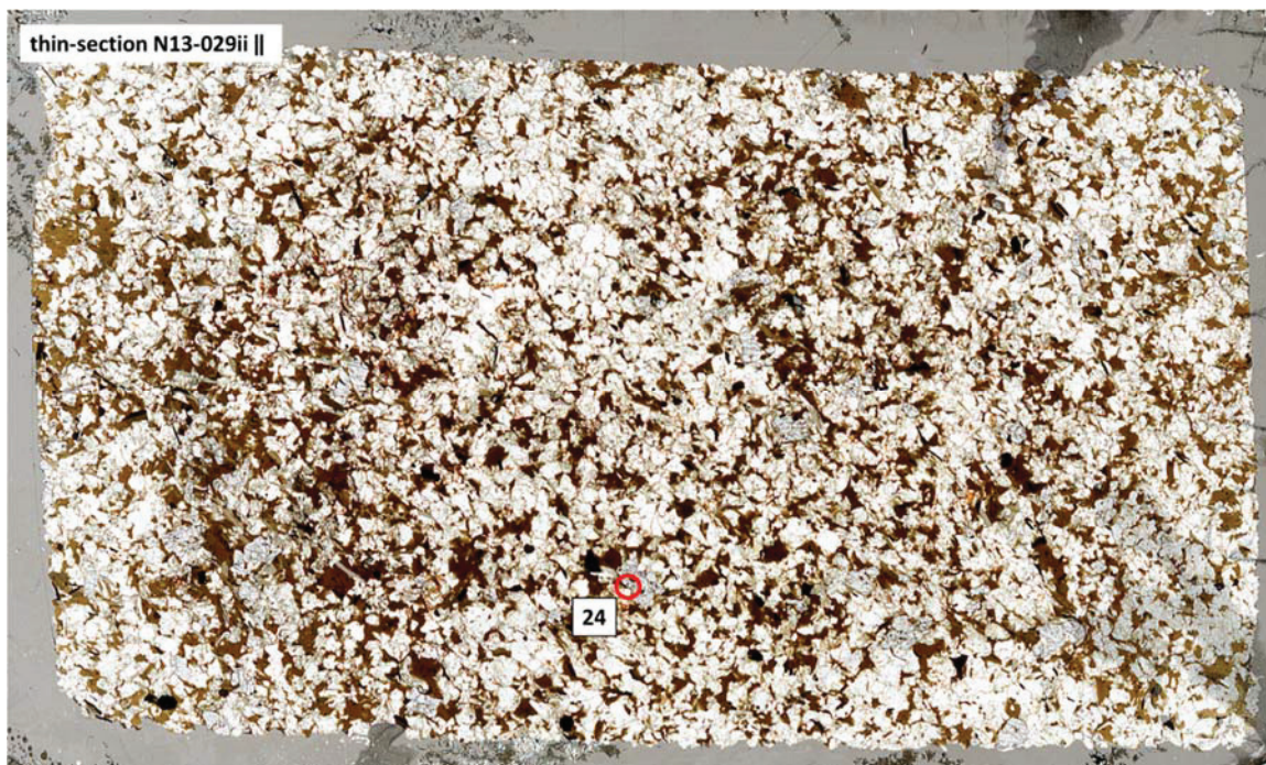
Figure D.3: Scanned polished thin section N13-029ii, parallel to foliation, with locations of an analyzed monazite grain.
