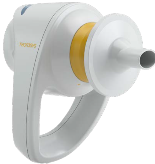
Figure 1.3: The hand held component of Thorasys tremoFlo™ with disposable anti-bacterial/anti-viral filter attached.
