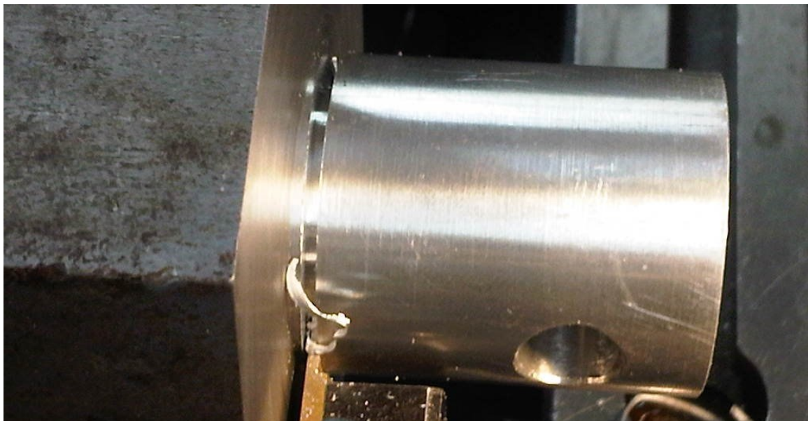
Figure 82 - Close-up of second face of angled groove being cut in cylinder.
