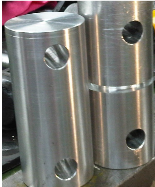
Figure 83 - Piston cylinders before (left) and after (right) grooves cut with angled groove jig.
