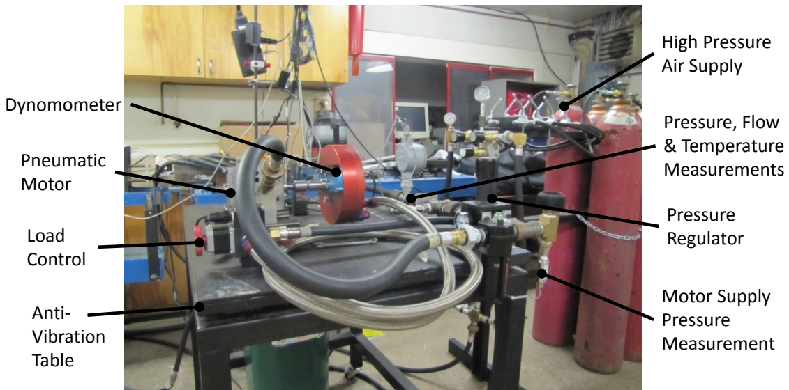
Figure 92 - Engine test setup.
