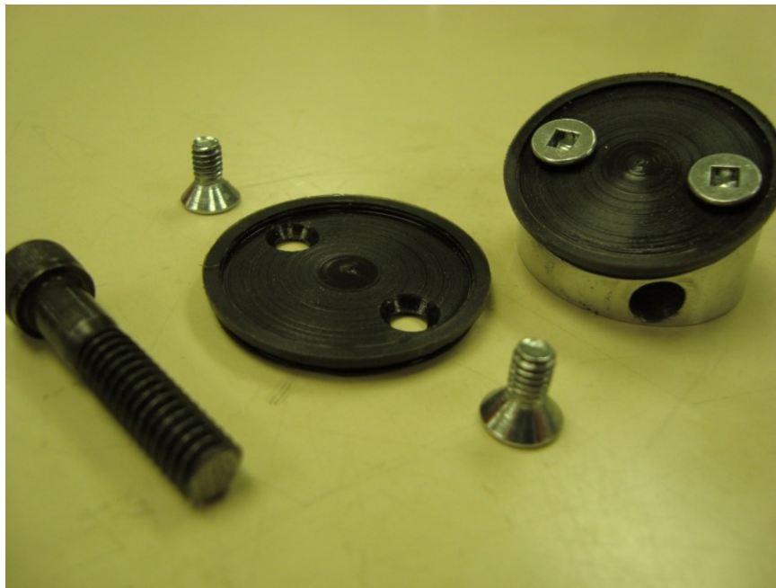
Figure 72– Three-piece piston assembly (80).
