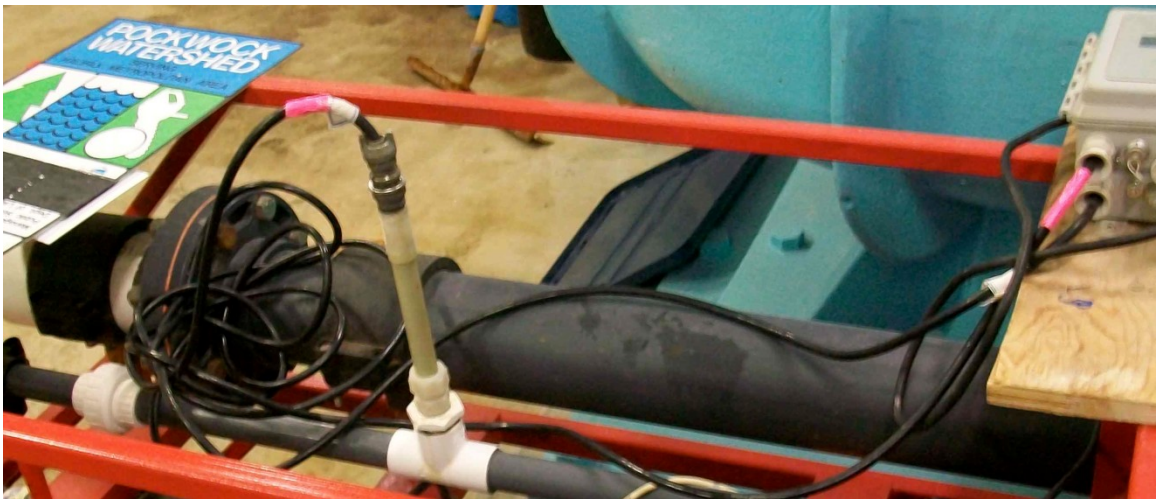
Figure 3.4 Close up of PVC test section of pipe loop
