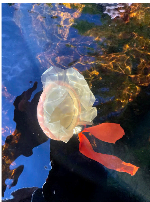
Passive samplers (SPATT) used to monitor the concentration of cyanotoxins in various watersheds across the region
