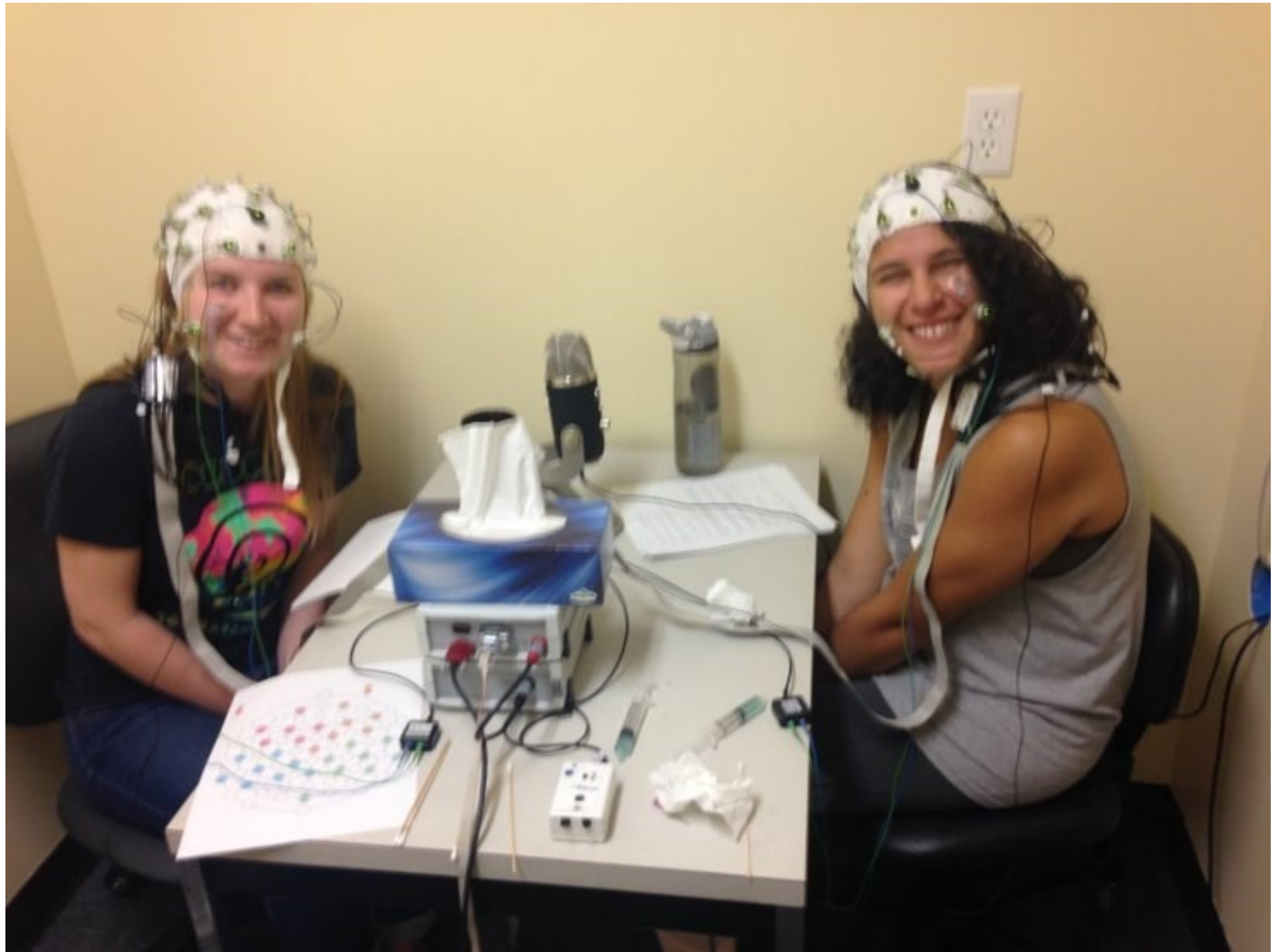
Fig. 1. An image of two participants using the EEG hyperscanning setup
