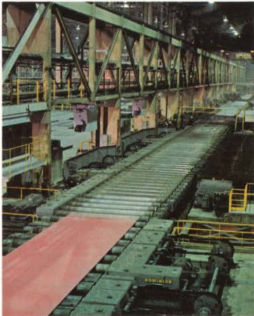
Rolled to a predetermined width and thickness for its specific purpose, the plate leaves the rolls on run-out tables.
