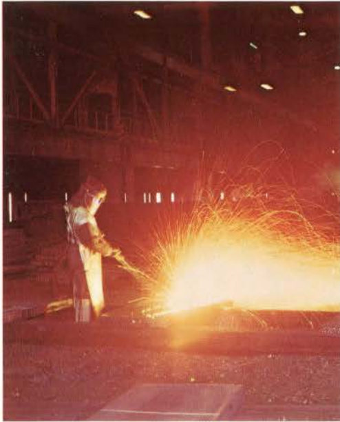
Steel slabs from the bloom mill are examined and any surface defects removed by 'scarfing' prior to rolling.
