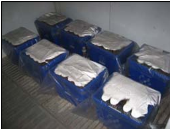
Cold test samples, during incubation at 10°C (D. Kerr)
