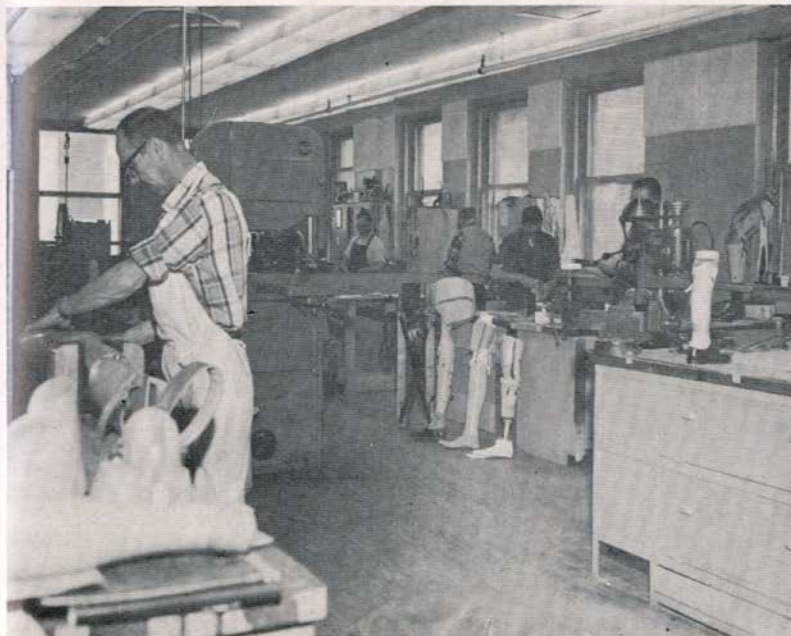
A view of the assembly shop. Note at the bench in the centre of the picture a Canadian hip disarticulation and a BK prosthesis ready for final fit and a BK socket with adjustable jig ready for the first fitting. On the bench in the right foreground is a child's patella tendon bearing appliance ready for finishing.
