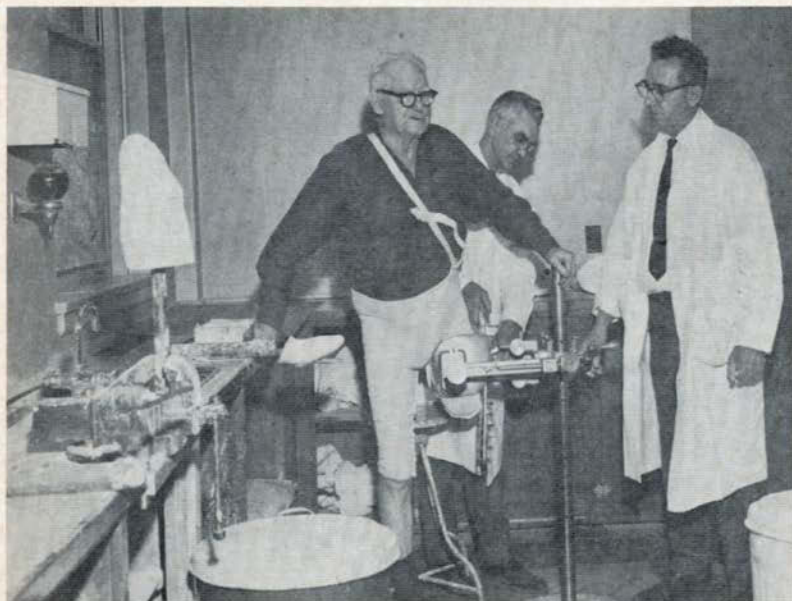
A view of the plaster room showing a patient being prepared for the VAPC casting jig. On the bench at left is a BK cast ready for modification and a BE arm cast.
