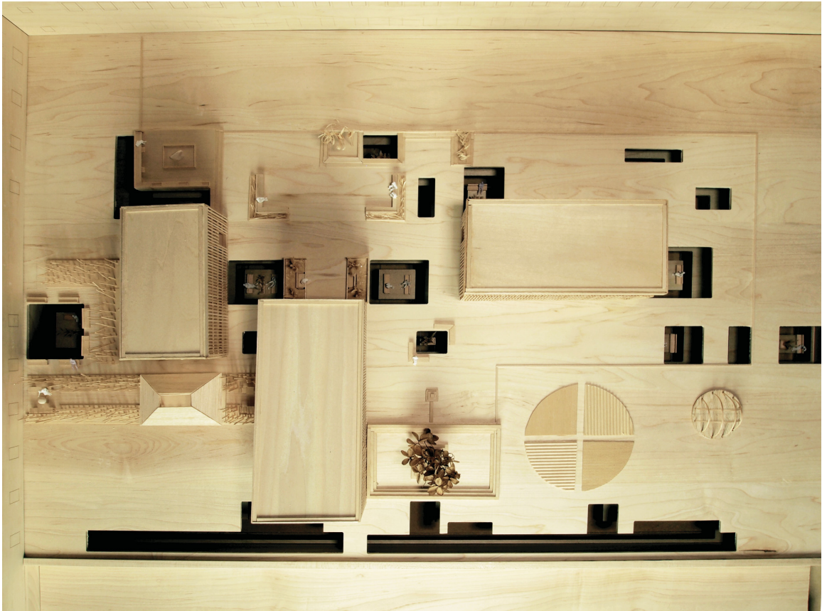
Figure 54. Top view of model. Note the garden spaces on the lower levels are inhabited and daylight can enter from above.
