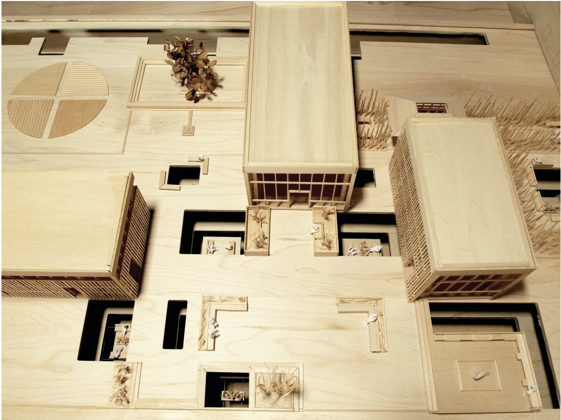
Figure 61. North view of the central step garden. Note the north facade glazing for indirect light to the cafe and wig salon.
