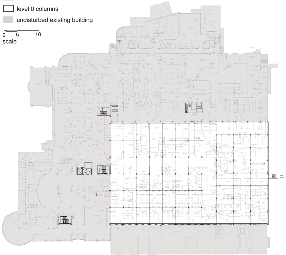
Figure 38. Level 0-1 column grid. (Modified plans of the existing Cross Cancer Institute, Edmonton, Alberta. 2010).
