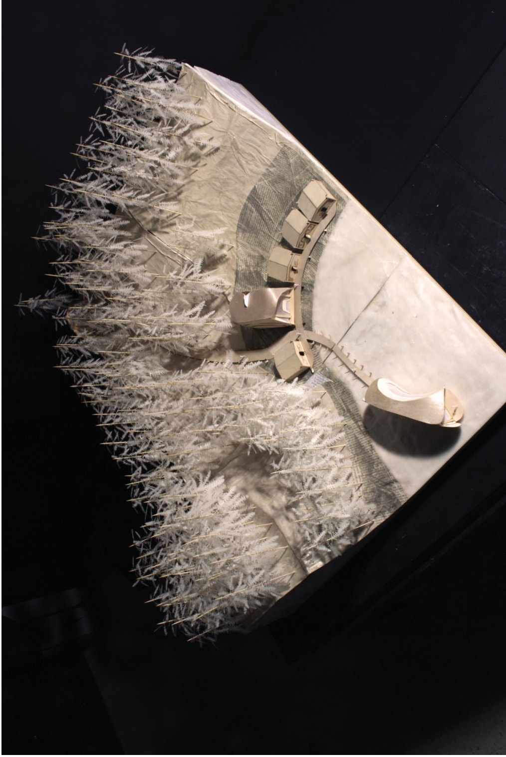
Fig.58: 1 to 100 site model. The buildings are placed within the site context. An elders cabin, executed in the same building language as the existing sleeping cabins is visible within the margin. A raised walkway connects all of the elements within the site.
