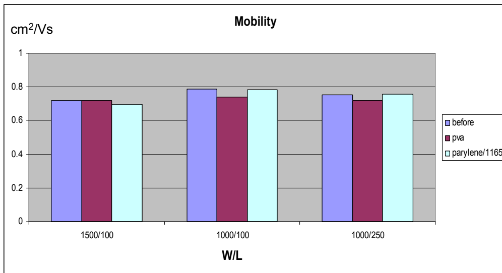
Figure 8.4 The mobility of pentacene devices after exposure to PVA-R, followed by parylene protection, and immersion in 1165.
