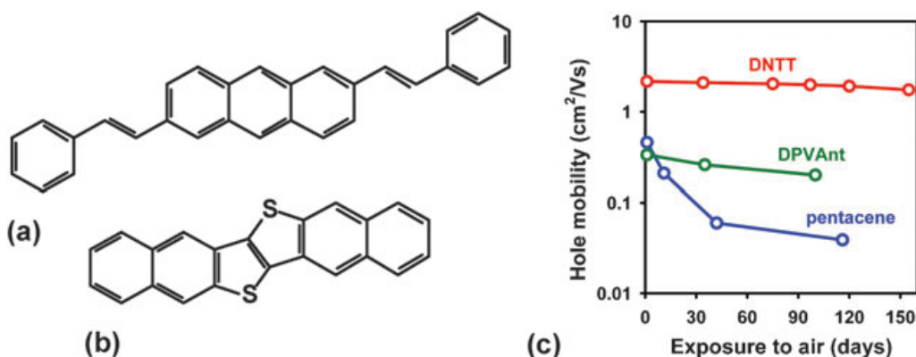
Figure 2.7 The improved ambient stability small molecule p-channel organic semiconductors. (a) 2,6-di[2-(4-phenyl)vinyl]anthracene (DPVAnt), (b) Dinaphtho-[2,3-b:2',3'-f]thieno[3,2-b]thiophane (DNTT), (c) Their mobilities degradation comparison with pentacene [2]. Reproduced by permission of The Royal Society of Chemistry.
