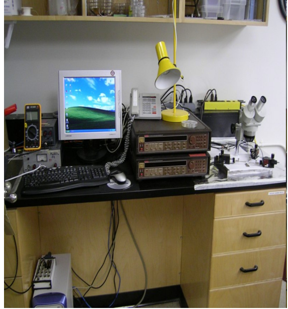
Figure 3.16 A probe station (left), and two SMUs (in dark brown, right).
