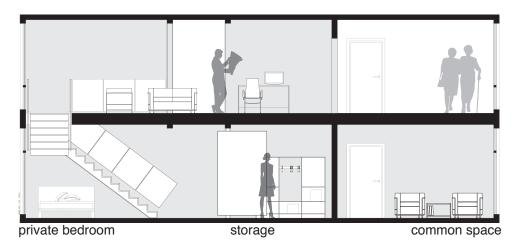
Figure 49: Vertical expansion of a studio apartment into a one bedroom.
