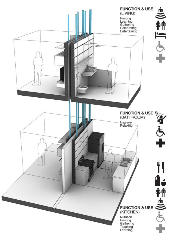
Figure 47: Sectional model, demonstrating the adaptability and flexibility of the service wall within a unit that accommodates multiple functions.
