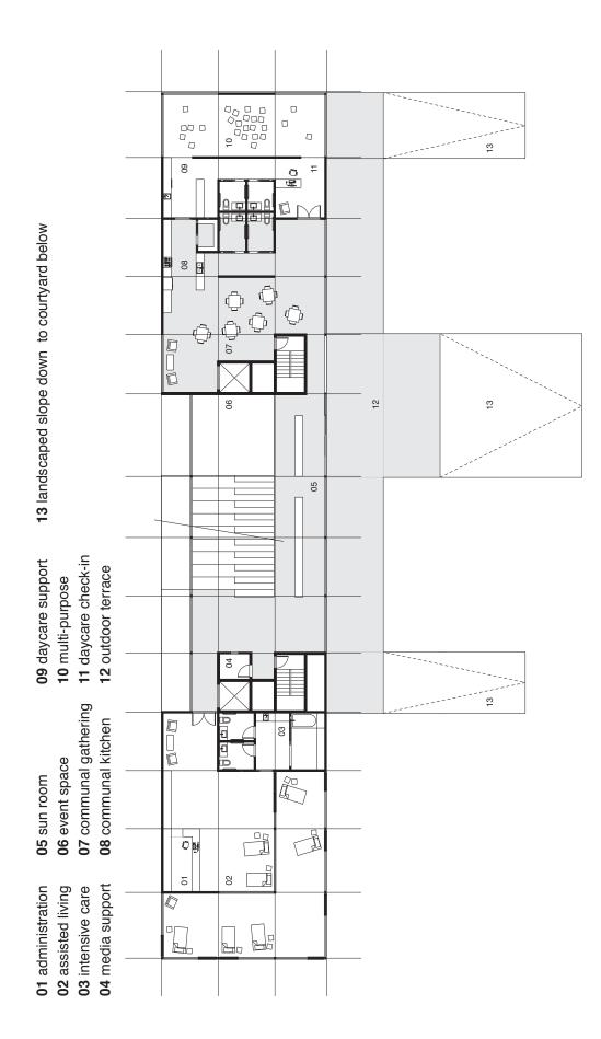
Figure 27: First floor plan, with care facilities (daycare, respite care, and assisted care) and the supporting programme (communal kitchen and dining area).
