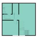
Figure 50: Partial upper floor plan, demonstrating how a single unit can grow and accommodate large families, allowing an extended family to exist within the same apartment while keeping their own space.
