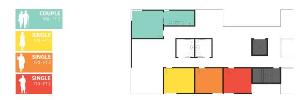
Figure 52: Partial upper floor plan, accommodating an elderly person with a live-in caregiver and a palliative care facility, where residents have a private room in addition to communal facilities.
