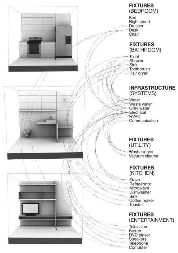
Figure 46: Sectional model. Analysis of overlapping building utilities in order to limit redundancy in HVAC, plumbing, and electrical infrastructure to allow a conversion of a space into a kitchen, bathroom, or living room
