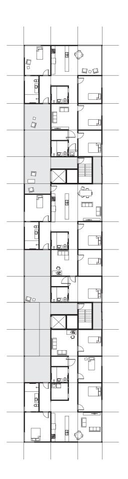
Figure 32: Typical upper floor plan. Variation 1: large apartments.
