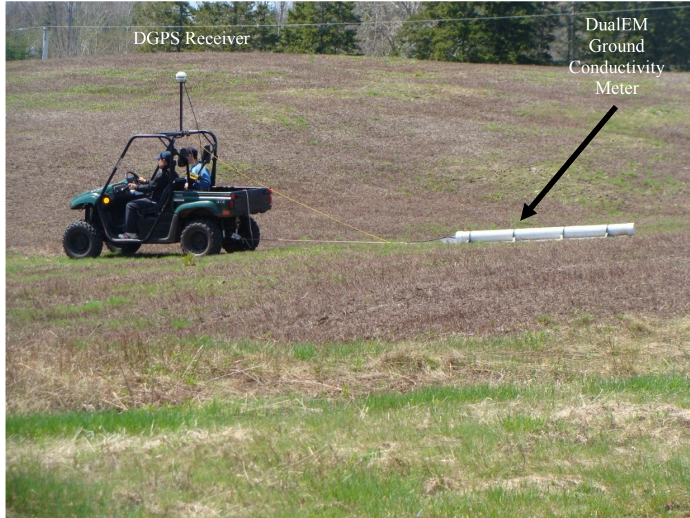
Figure 3-1. Measurement of ground conductivity using DualEM.
